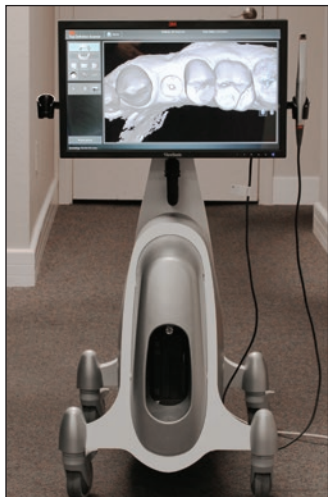
Figure 1. Chairside intraoral optical impression scanner (True Definition Scanner [3M ESPE]).
