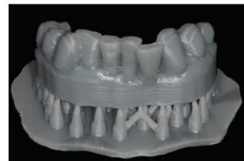
Figure 20. The STL file was uploaded to the printer and a 3-D printed model was fabricated (Form 1+).
