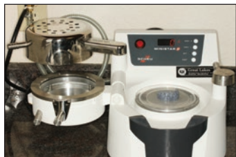
Figure 21. The supports were removed and the model was processed with isopropyl alcohol. The model was placed in a vacuum-forming machine (MiniSTAR S [Great Lakes Orthodontics]) and a sheet of polyethylene was vacuum formed over the model (Bioplast [Great Lakes Orthodontics]).
