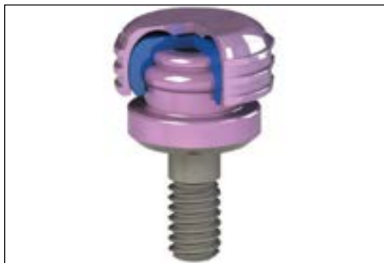
Figure 3. Contemporary stud-style attachment systems, such as LOCATOR R-Tx (ZEST Anchors), have designs that permit dual retention, increased resiliency to accommodate significant angulation, low profile heights, low hygiene maintenance, and a pink Titanium Carbon Nitride coating that reduces wear.
