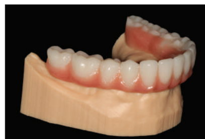
Figure 9. A 3-D printed prototype prosthesis was fabricated from dental resins (NextDent C&B MFH and NextDent Denture 3D+ [3D Systems]) and joined together in the dental laboratory.
