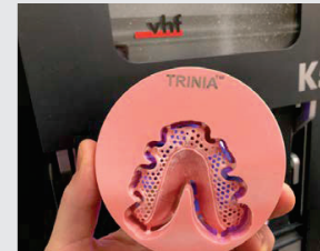
Figure 5 —The design of a maxillary overdenture framework was outsourced to a design center (FullContour), placed into a CAD/CAM milling system (K5, VHF) and milled using a fiber-reinforced composite polymer (TRINIA, Bicon Dental).
