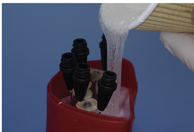
Figure 15. Casting of polyvinyl siloxane material. Note air inclusions eliminated by pressurized polymerization.
